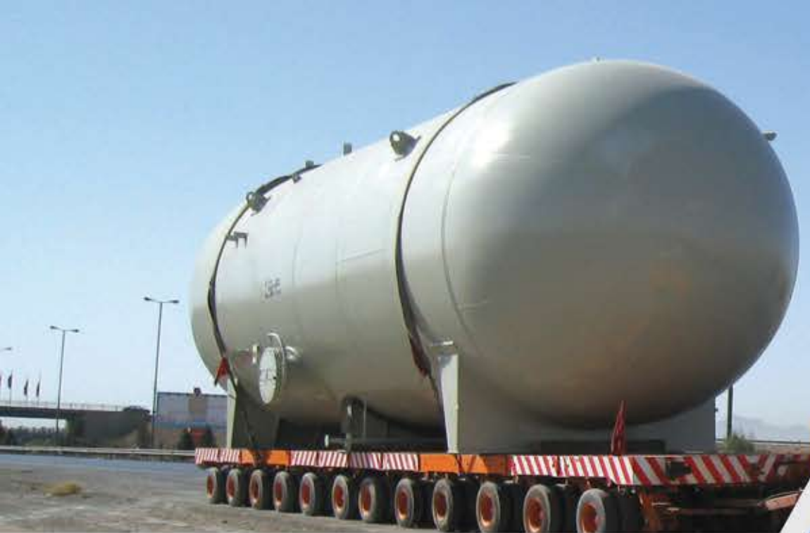
PURGE GAS VESSEL
