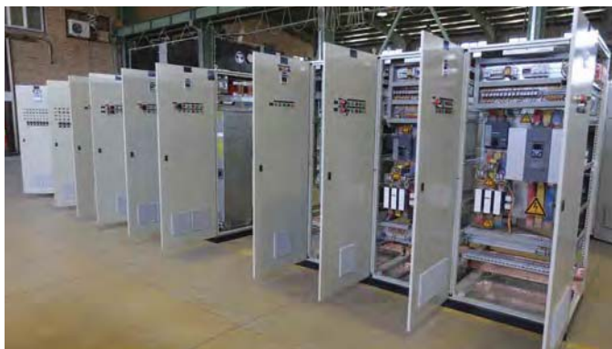
MCC Panel With VFD & Soft Starter
