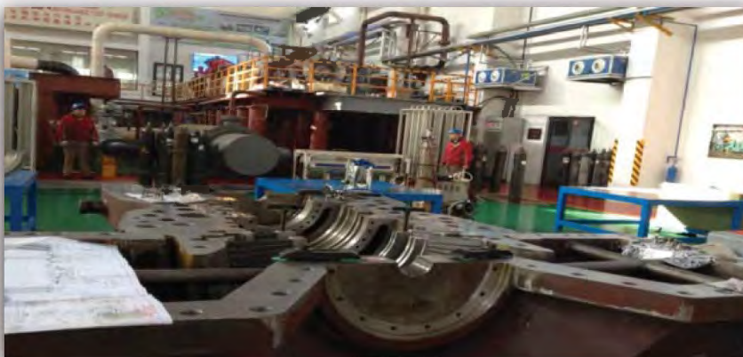
NH3 Refrigeration Compressors (LP/HP) c/w Mechanical Drive Steam Turbine
