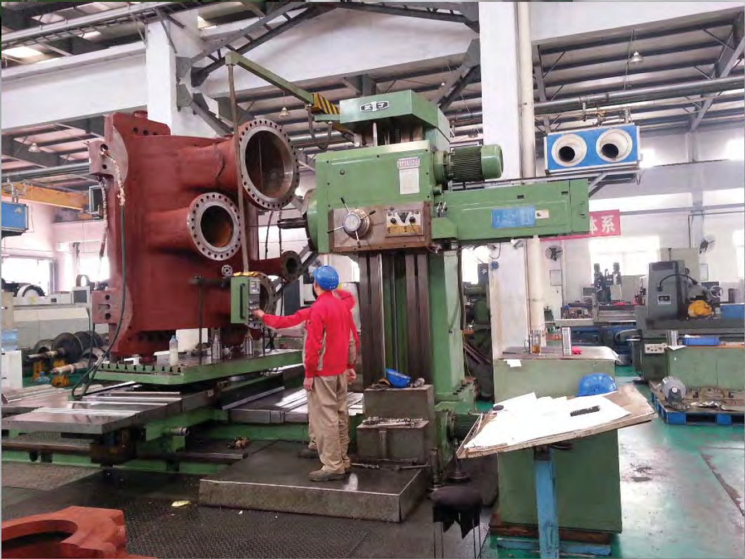
Compressor Casing Machining
