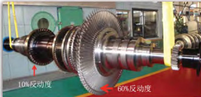
NEW JCM Advanced Impulse Type Rotor
