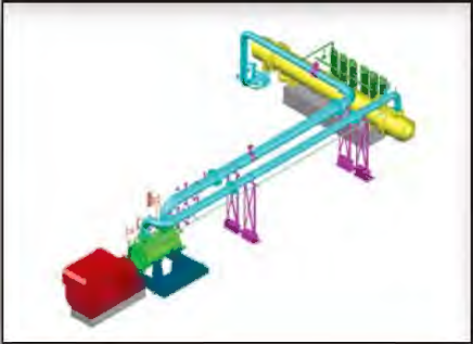
Syngas compressor ASME PTC10-2 Shop performance test bed design
