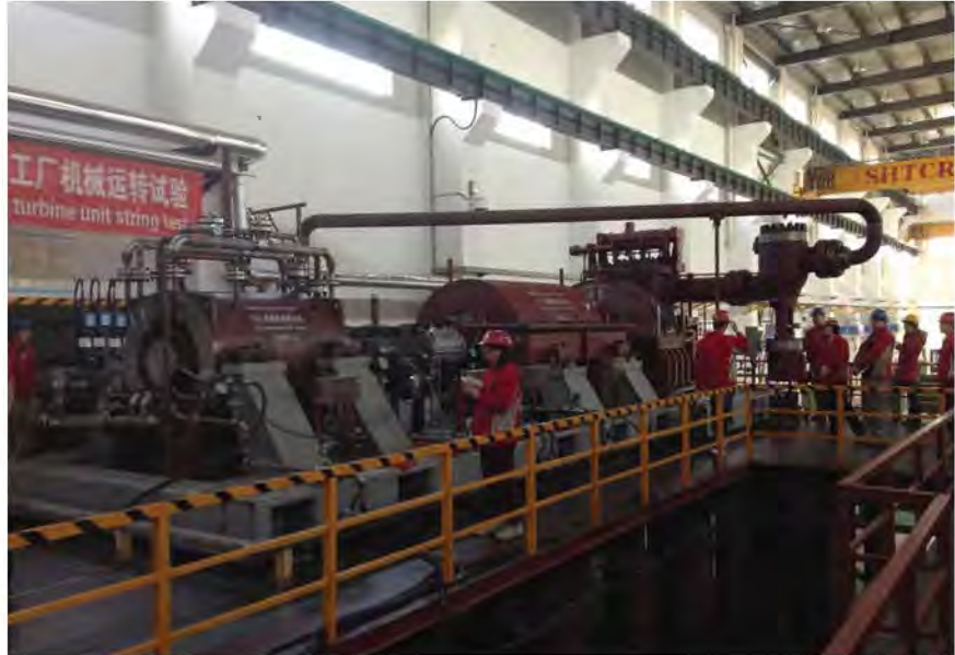
A large-scale CO2 compressors (LP/HP) + Gear Box + Steam Turbine Train in the String Test.
