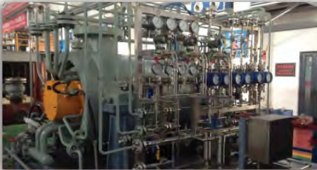
Sales Gas Compressors c/w Dry Gas Seal Control Panel on Skid
