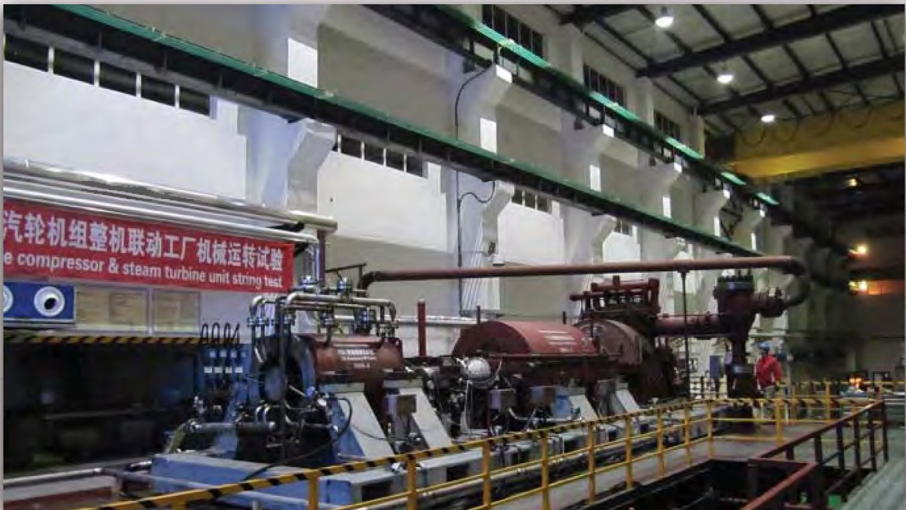
String Test of of CO2 Train: Steam Turbine – LP Compressor- Gearbox- HP Compressor
