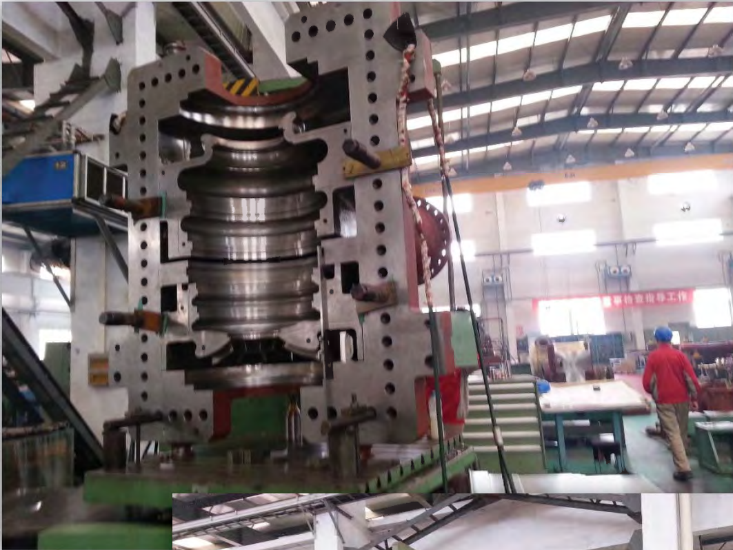
Turbine Casing Machining
