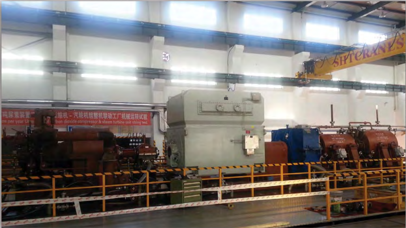
String Test of Complicate train: Including 6 equipment Steam turbine-Gearbox-VFD Motor-Gearbox-LP compressor –HP Compressor
