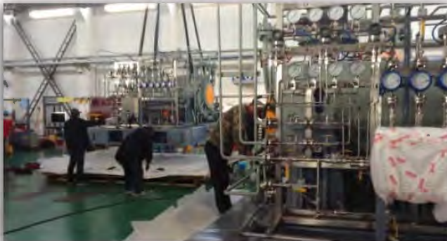
Sales Gas Compressors c/w Dry Gas Seal Control Panel on Skid
